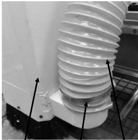
Dust shroud Clamp Dust hose
