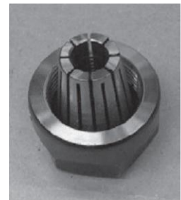
Collet fitted to spindle nut
