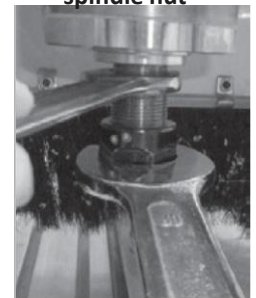
Tightening the spindle nut
