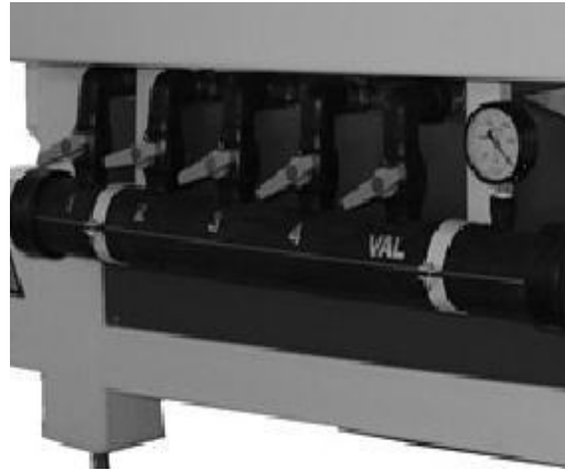
Vacuum zone on / off switches
