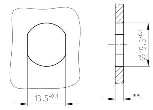
Installation recommendation only valid for housings with bevels (anti-twist protection)!
