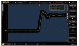
User defined mask, Pass/Fail counts, stop on fail, fail alarm
