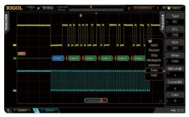
Built-in dual-channel 25 MHz source (MSO/DS2000A-S)
